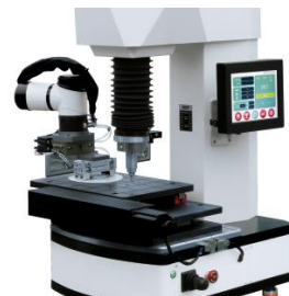
The robot automatically places the workpiece on the hardness tester station for automatic measurement
